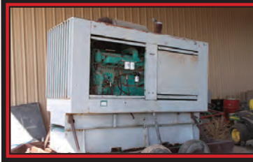
Generator 150 KW w/12 Wire. Could be wired 3-Phase or 240 or 480, 3-Phase Allis Motor on Trailer
