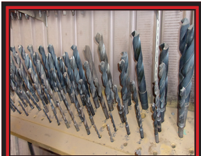
Appx 50 Drill Bits - 1/2" - 1 1/2" w/Morse Taper Shank
