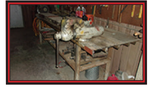
Hyd Jacks, Pipe Wrenches, Bolt Cutters, 3'x10' Channel Iron Shop Table w/Dayton Grinder & Wilton 8" Vise
