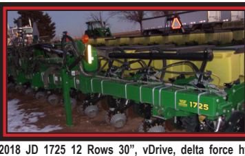
2018 JD 1725 12 Rows 30", vDrive, delta force hyd down pressure, Vapilly fertilizer system, Martin row cleaners with cleansweep, 2020 Monitor, used approx. 2000 acres, Stack Fold, Very Clean
