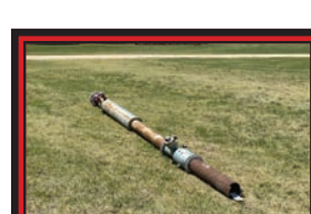
6' cooling coil with chem valve
