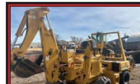
Vermeer V-4150 ditcher backhoe, rebuilt pump, new chain & sprockets
