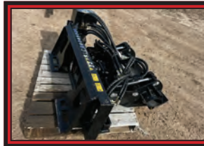
New Skid-Loader Pipe Grapple
