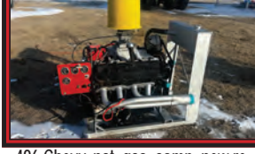
496 Chevy, nat. gas, comp. new rebuilt conv to dstrbr in flat top lifters
