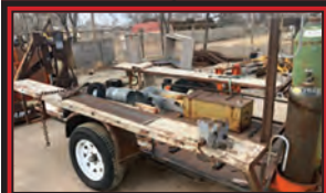
Shop-built Welding Trailer
